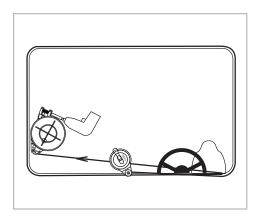
Step 1: Cut the adhesive bead from the starting point to the bottom right corner.
