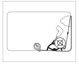
Step 4: Cut the left A-pillar downwards to the starting point.
